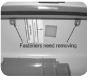
The internal plastic frame is held in place with eight connectors (two connectors on all four sides). A combination of plastic pins and nut/screw fasteners are used to secure the frame.
