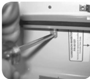
If the pins are flat, use a screwdriver to tap them out through the enclosure wall.
