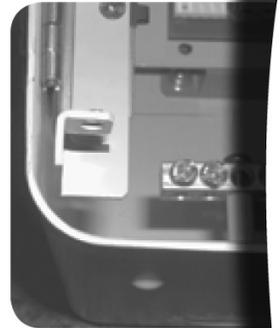
Correct orientation of left sider adapter
