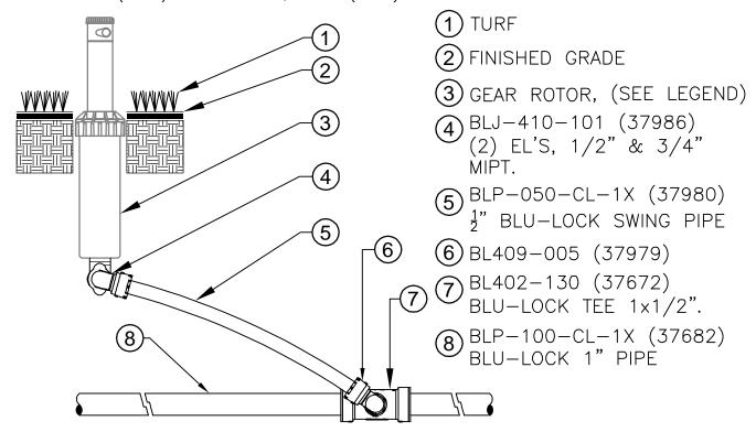
INSTALL POPUP SPRAY SPRINKLER PLUMB TO FINISHED GRADE AND 4" FROM PAVED EDGE, BUILDINGS AND FENCE AREAS, AND INSTALL FLUSH TO GRADE, ADJUST COVERAGE TO AVOID OVERSPRAY ONTO PAVED SURFACES, FENCES, BUILDINGS AND PARKING LOTS.
