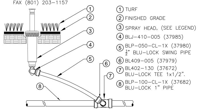
INSTALL POPUP SPRAY SPRINKLER PLUMB TO FINISHED GRADE AND 4" FROM PAVED EDGE, BUILDINGS AND FENCE AREAS, AND INSTALL FLUSH TO GRADE, ADJUST COVERAGE TO AVOID OVERSPRAY ONTO PAVED SURFACES, FENCES, BUILDINGS AND PARKING LOTS.
